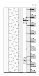
The gap between cladding battens must be equal to or greater than 20 mm wide to allow fixing pre-assembled facade modules to the structure.
