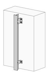
Fixing through a system of metal fastening brackets that allows adjusting the position of the battens regardless of the support wall flatness.
