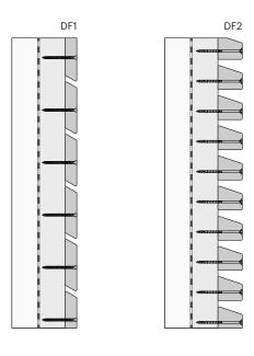
In horizontal battens cladding, profiles with a sloping top edge to allow water drainage and prevent dirt accumulation are recommended.
