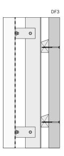
In open joints installation, the gap between battens must be equal or greater than 8 mm wide to avoid moisture traps. [See DF1].
