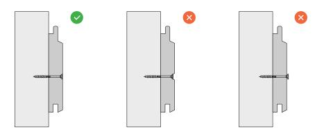
• Use one fixing at each cladding/batten intersection when the cladding profile is <140 mm wide. Use two fixings when the cladding profile is >140 mm wide. Always respect the edge distances recommendations.
