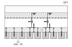
The gap between cladding battens must be equal or greater than 10 mm wide to allow fixing pre-assembled facade modules to vertical support battens.
