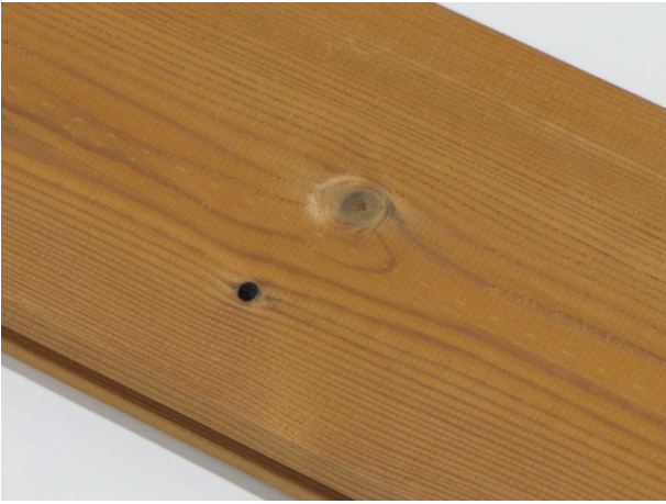
Small knothole (not throughout) on a board is allowed.
