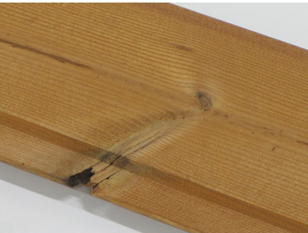
Defects which are invisible after installation are allowed.
