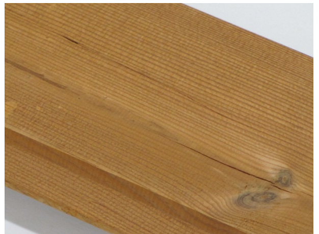
Small shakes on the surface are allowed.
