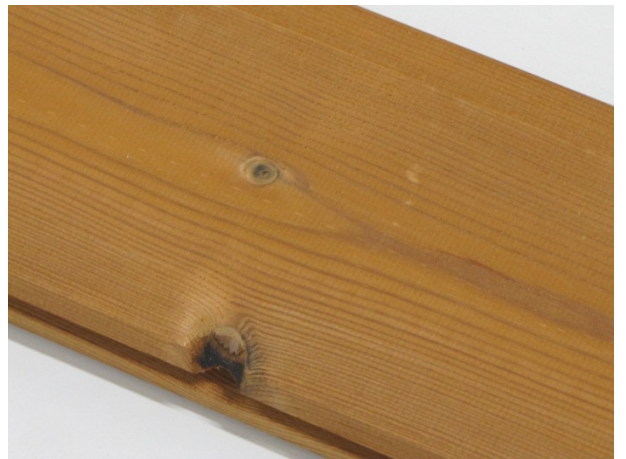
Small missing knot on the edge is allowed.
