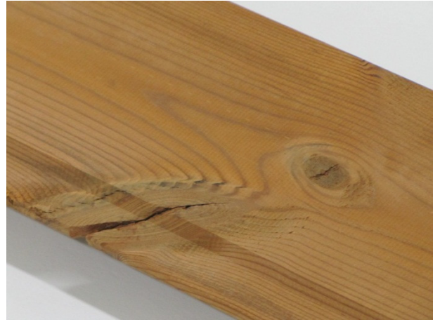
Single crack of a knot is allowed.
